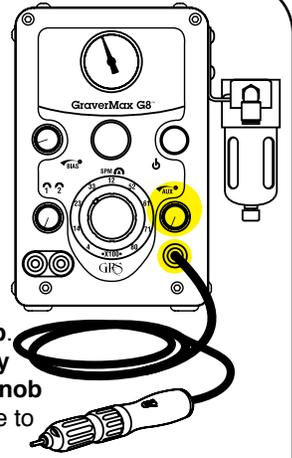
*SPECIAL NOTE: When using the NSK High Speed Handpiece do not exceed 2.5bar (35psi).*
